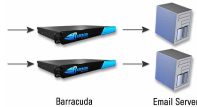
Figure 3: Level 3 Redundancy Setup
